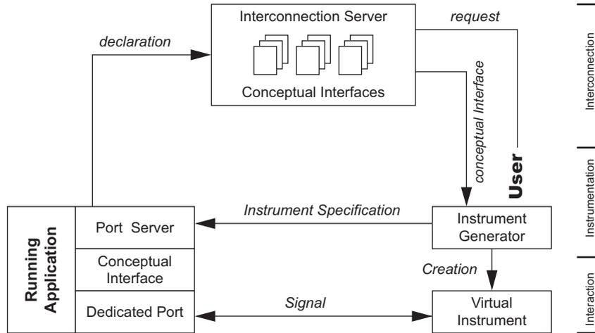
Figure 5.3: **Focale** defines three functional levels: (1) interconnection, where the interconnection server is used, (2) instrumentation, aiming at the user interface building and adaptation, and (3) interaction, where the final exchanges between user and application actually take place.
