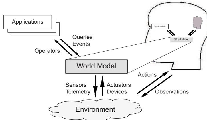
Figure 1.2: **Sentient Computing.** Using sensors and resource status data to maintain a model of the world which is shared between users and applications.
