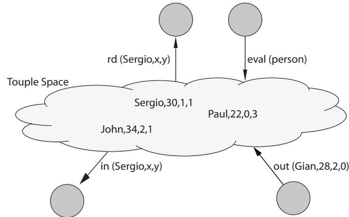
Figure 1.4: **Tuple Space abstraction.** Tasks can generate asynchronous requests to read, take, write and eval tuples.
