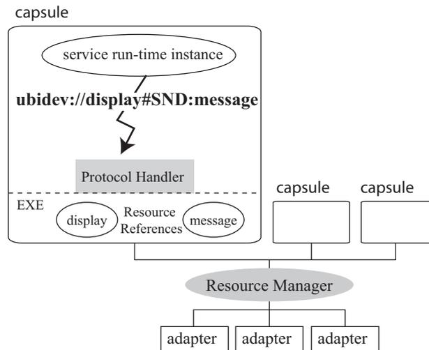
Figure 3.3: **UBIDEV protocol handler.** *The consistence of the mapping between concepts and resources reference is evaluated inside the service execution environment by the protocol handler.*
