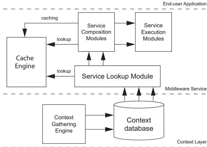
Figure 5.2: **CB-SeC**. *Three layer architecture.*
