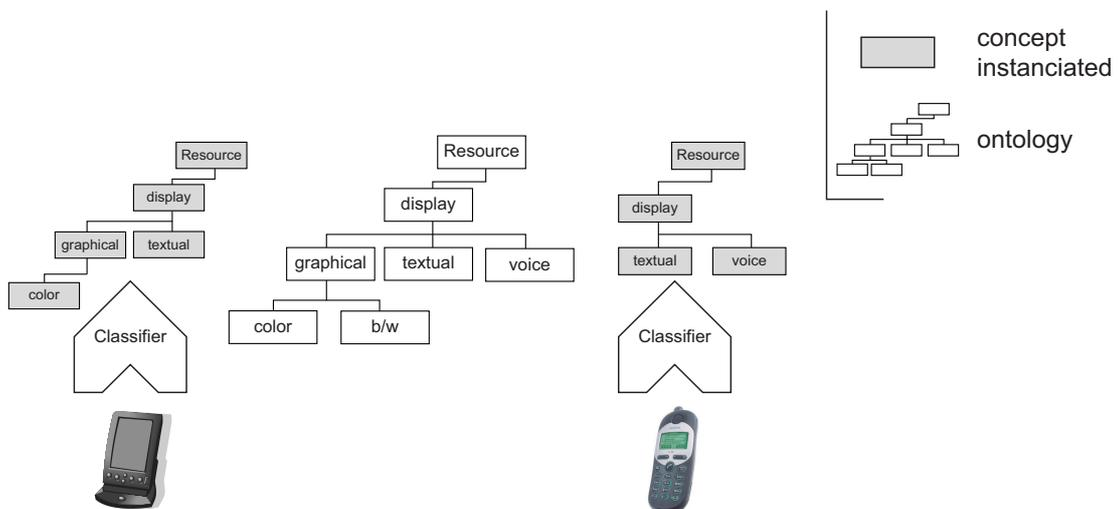
Figure 2.5: **UbiDev Classification Process.** *An example of classification of physical resources. Classifiers are seen as the knowledge required to identify the relation between the icons in the symbol system and the physical elements.*
