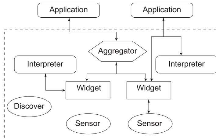
Figure 1.3: **Context Toolkit.** An interaction example between applications and Widgets and between Interpreters and Aggregators.
