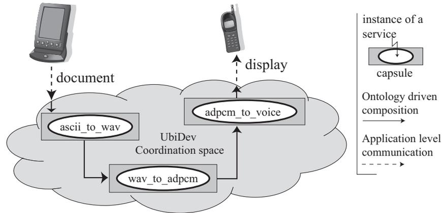
Figure 4.3: **Ubiquitous Message System.** *The application can compose capsules in a more structured entity, a composite high level service (document\_to\_display).*
