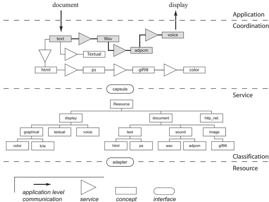
Figure 4.1: **Ubiquitous Message System.** A composite service can be realized by the coordination manager by composing existing services according to the classification of the underlying environment. Coordination manager solves user tasks by finding the path from the input resource generating the output resource. This path represents a service invocation chain. Service manager takes in charge the service execution process.
