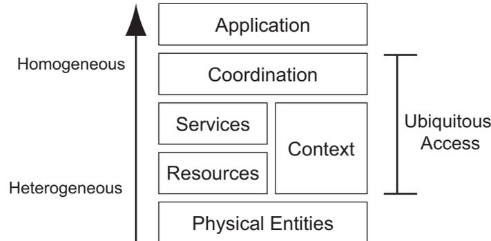
Figure 2.4: **UBIDEV reference model.** UBIDEV separates the coordination aspects from the resource and service management in order to hide at the application level the heterogeneity of the underlying environment.
