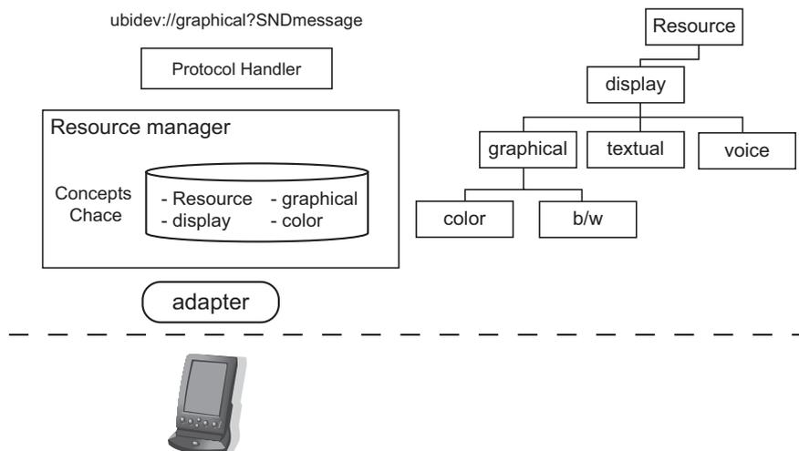
Figure 3.2: **UBIDEV Resource Abstraction.** *The virtual representation of a physical entity inside UBIDEV is composed of an adapter containing the specific resource access information, of the result of the classification process that allow to abstract the resource according to the application ontology and of the access protocol that grant the consistence of the mapping between concepts and resources.*
